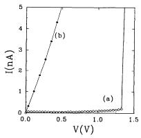
Fig.6 Typical I-V characteristics of the NBPDA film of (a) the unrecorded region and (b) the recorded region by STM.
