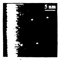
Fig.5 A  $28 \times 28 \text{nm}^2$  STM image on NBPDA thin film with recorded marks by applying pulse voltage of 4V for 2ms.  $V_b$ =0.10V,  $I_t$ =0.19 nA.
