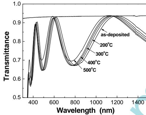
Fig.4: Transmittances of the ZnS films annealed at different temperatures at the wavelength from 300 to 1500 nm
