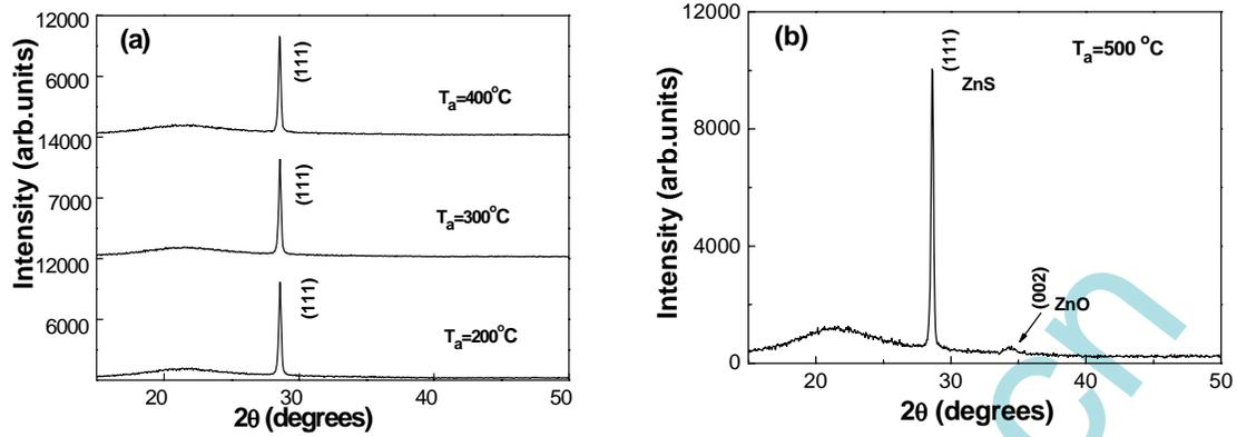
Fig.2: X-ray diffraction patterns for ZnS films annealed (a) at 200, 300 and 400 °C, (b) at 500 °C, which were deposited at 200 °C
