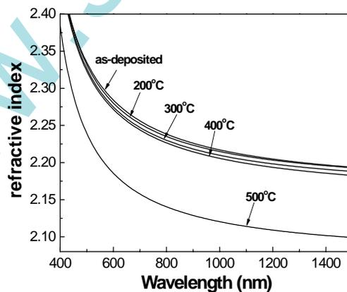
Fig.5: Refractive indices as a function of wavelength of ZnS films annealed at different temperatures
