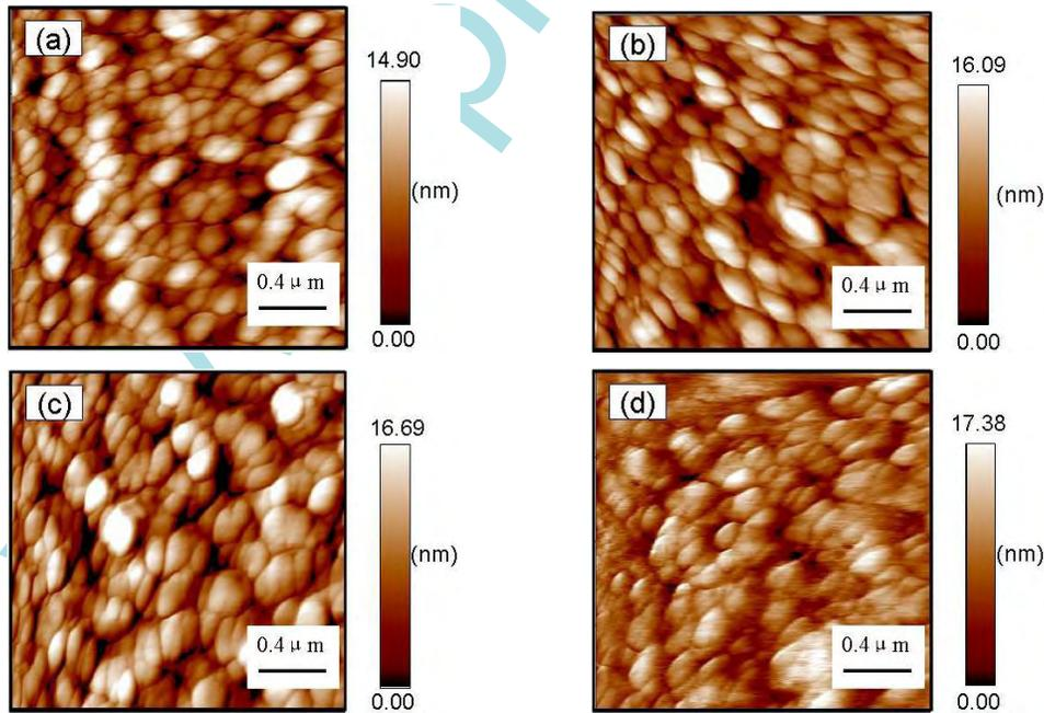
Fig. 3: Surface morphology of the ZnS film annealed at 200,300,400,500 °C respectively
