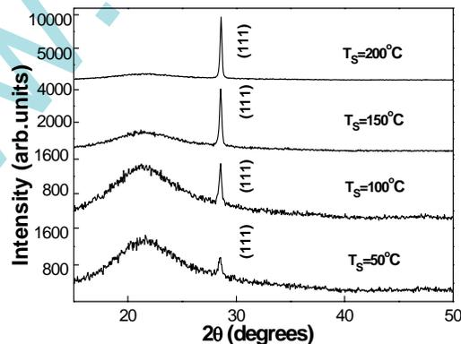
Fig.1: X-ray diffraction patterns for ZnS films deposited at different substrate temperatures
