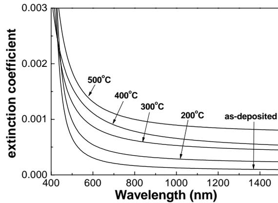
Fig.6: Extinction coefficients as a function of wavelength of ZnS films annealed at different temperatures
