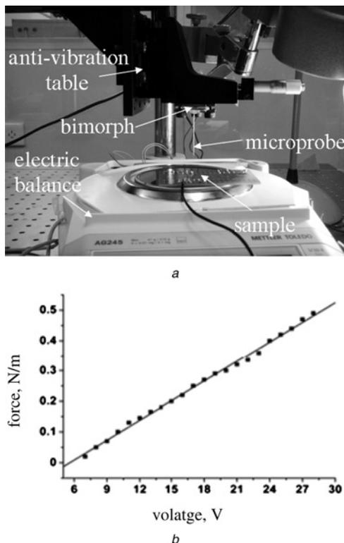
Figure 8 Properties of piezoelectric microcantilever
