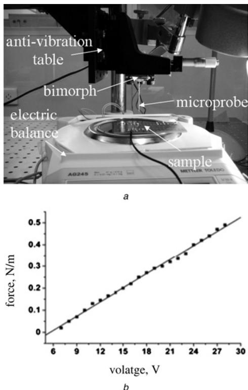
Figure 8 Properties of piezoelectric microcantilever
