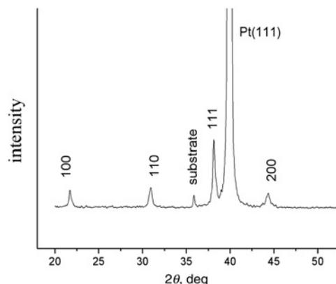
**Figure 5** XRD pattern of the PZT thin films
