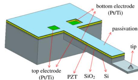
Figure 1 Schematic diagram of the piezoelectric microcantilever probe
