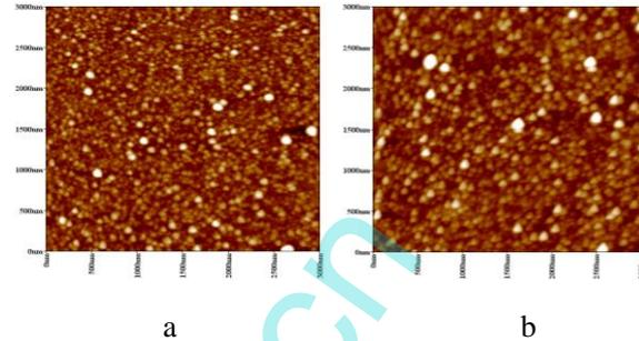
Fig.5 AFM images of SiO<sub>x</sub> coatings on glass substrates with input power (a=1500 W, b=2000 W)
