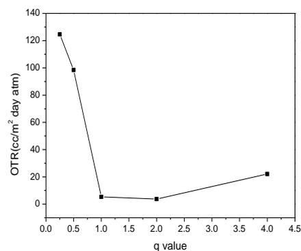
Fig. 2 OTR of about 60 nm thick SiO<sub>x</sub> coated PET (12.5 μm) for various ratio of gas fluxes at plasma condition of
