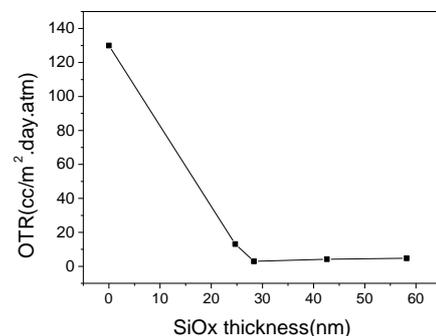
Fig.9 OTR of SiOx films coated PET for various films thicknesses at plasma conditions  $q=2$ ,  $p=20$  Pa,  $P=2000$  W,  $t_{on}=4$  ms and  $t_{off}=40$  ms
