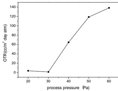
Fig.6 OTR of about 60 nm thick SiOx films coated PET (12.5um) for various working pressures at plasma conditions of  $q=2$ ,  $P=1500$  W,  $t_{on}=4$  ms and  $t_{off}=40$  ms.
