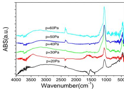
Fig.7 FTIR Spectrum of SiOx coatings at various working pressures (from 20 Pa to 60 Pa)
