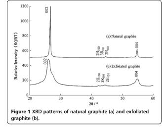
controlled timer and intensity was used for irradiation. About 5 g of pristine natural graphite flakes was mixed with the volume ratio (1:30) mixture of concentrated nitric acid (98%) and hydrogen peroxide (30%). Then the resulting mixture was ultrasonicated, stirred for 1 h, and washed using diluted nitric acid (30%). A spot of acetic acid (CH<sub>3</sub>COOH, about 6 ml) was added to the reactant
