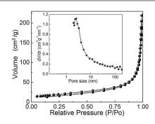
Fig. 3  $N_2$  adsorption–desorption isotherms of CoHPO<sub>4</sub>·3H<sub>2</sub>O ultrathin nanosheets, and the inset shows the pore-size distribution curve.
