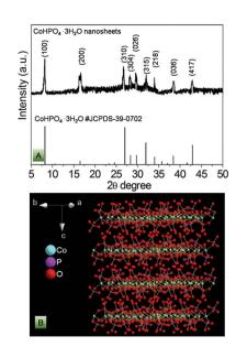
**Fig. 1** (A) XRD patterns of as-prepared samples and JCPDS-39-0702; (B) the schematic crystal structures of  $CoHPO_4 \cdot 3H_2O$  super cells (2  $\times$  2  $\times$  2 slabs) projected based on data of ICSD-86668.
