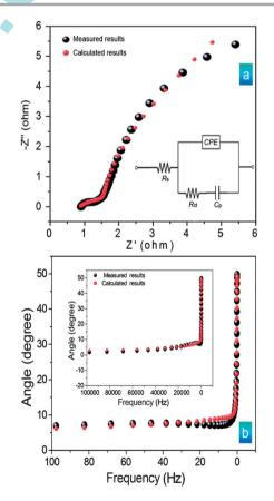
**Fig. 5** The electrochemical impedance spectra (EIS) of the electrodes at room temperature and its corresponding calculated curve, in insets of (a) the equivalent circuit for the electrochemical impedance spectrum; and (b) the phase angles for impedance plots and its corresponding calculated curve.
