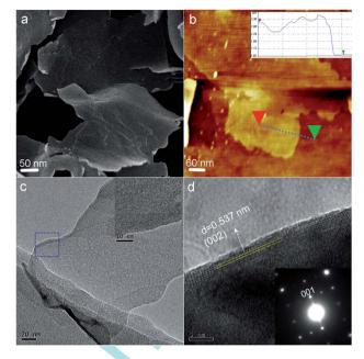
**Fig. 2** (a) SEM image of as-prepared  $CoHPO_4 \cdot 3H_2O$ ; (b) AFM image; (c) TEM image; (d) HRTEM image from the magnification of the section marked in (c) and its corresponding SAED pattern.
